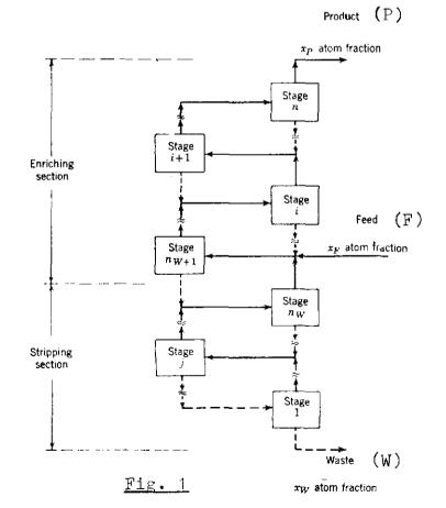
and waste end is called the <u>stripping section</u>, used to increase the recovery of the desired isotope from the feed. Stages of the cascade are numbered consecutively from 1 at the waste end of the plant to n at the product end. The highest stage of the stripping section is numbered  $n_{\rm W} \cdot$
